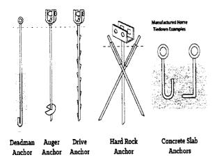
Tie down anchors shall be installed in accordance with the anchor manufacturer's specifications.
